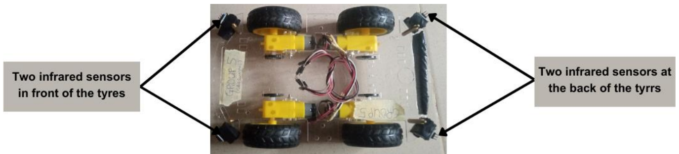
Fig. 10. Top view showing the mounted infrared sensors on the chassis.
