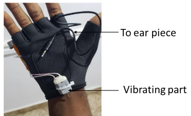
Fig. 11. Glove housing the motor for vibration mode.
