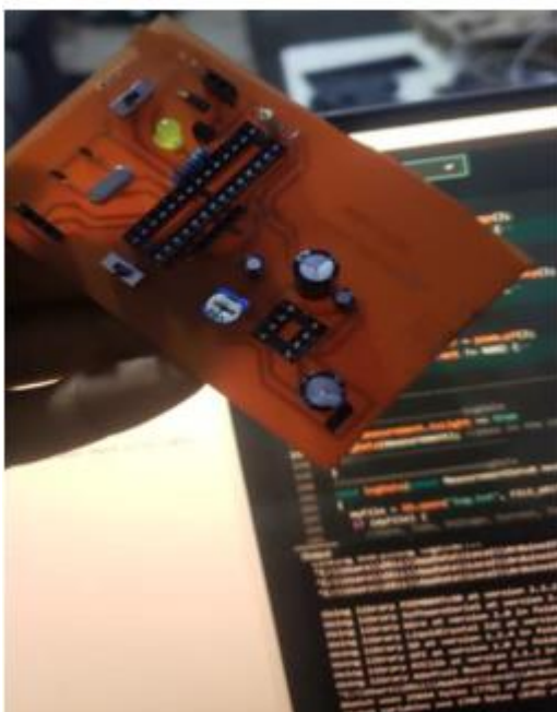
Fig. 9. Component placement on the fabricated PCB.
