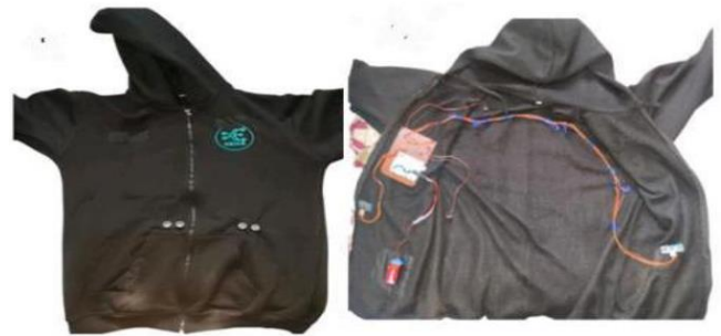
Fig. 3. Ultrasonic sensor-based assistive navigation jacket.
