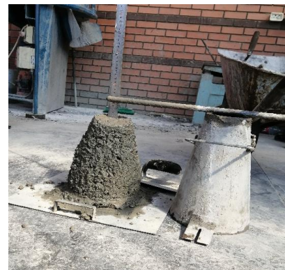
Fig. 3: Slump test set-up
