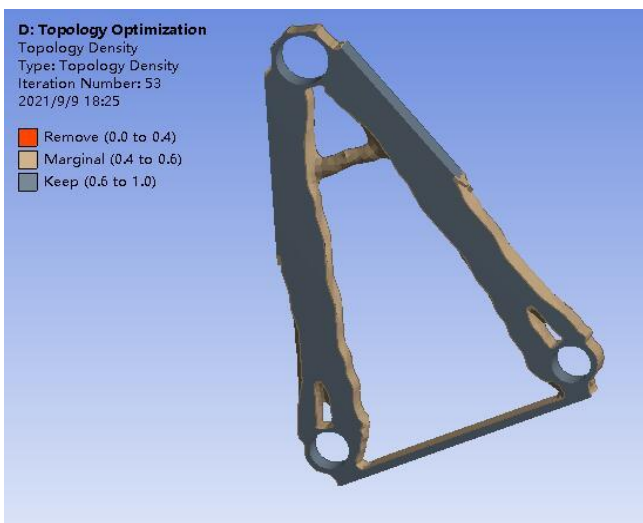
Fig. 2. Topology optimization cloud diagram of suspension arm
