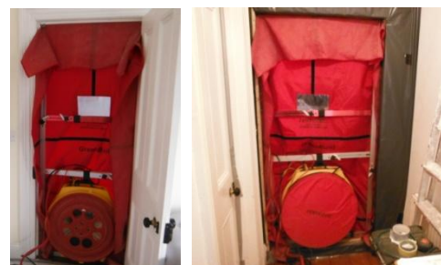
Fig. 3. Image of air blower fan inserted in internal door opening (room 1) and in frame at bottom of stairs (room 2).
